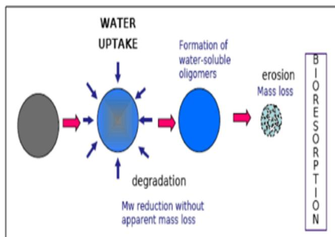
Figure 5: Drug release mechanism from Biodegradable polymer system
