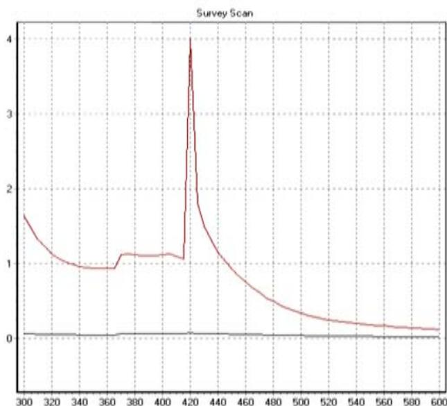
Fig 2: UV-Vis spectroscopy analysis of silver nanoparticles at 420 nm
