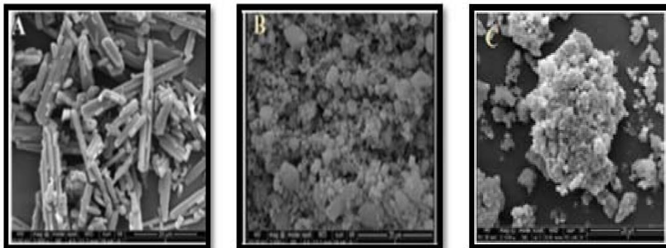
**Fig 2: SEM images of A) Ramipril B) Sylysia FCP 350 and C) S-SNEDDS**
