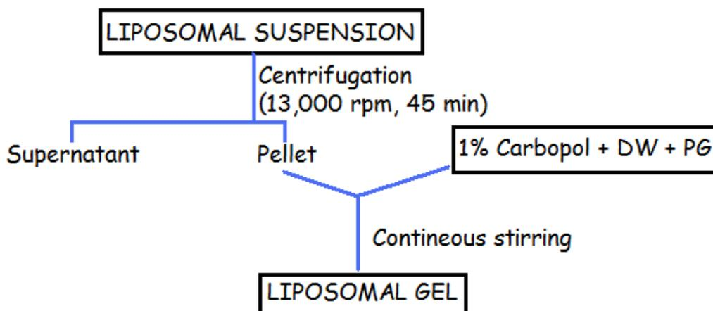
Fig 2: Schematic Representation of Preparation of Liposomal Gel
