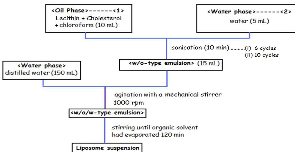
Fig 1: Schematic Representation of Preparation of Fluconazole loaded Liposomal suspension by MCV method
