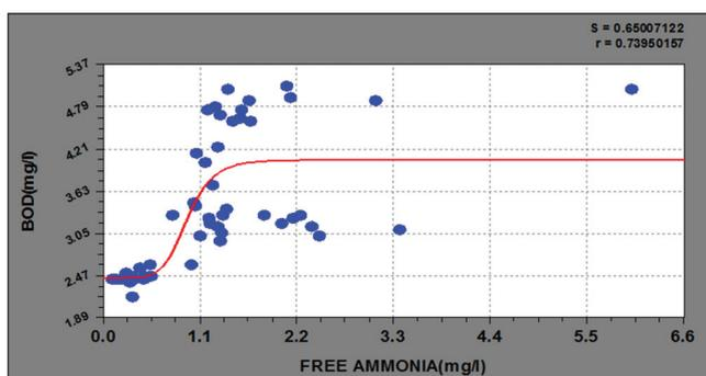
**Figure 7:** MMF model fit showing the mathematical relationship between free ammonia and biochemical oxygen demand
