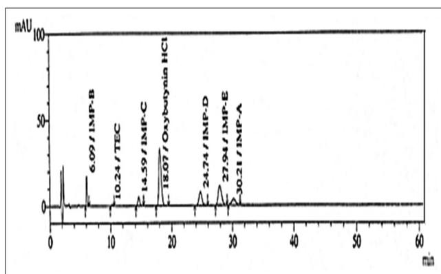
Figure 3: Chromatogram of known impurity mixture with oxybutynin HCl
