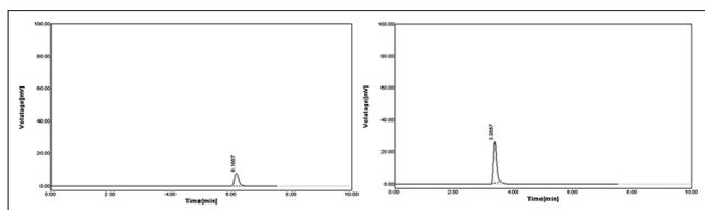
**Figure 2:** Chromatogram of ursodeoxycholic acid and silymarin
